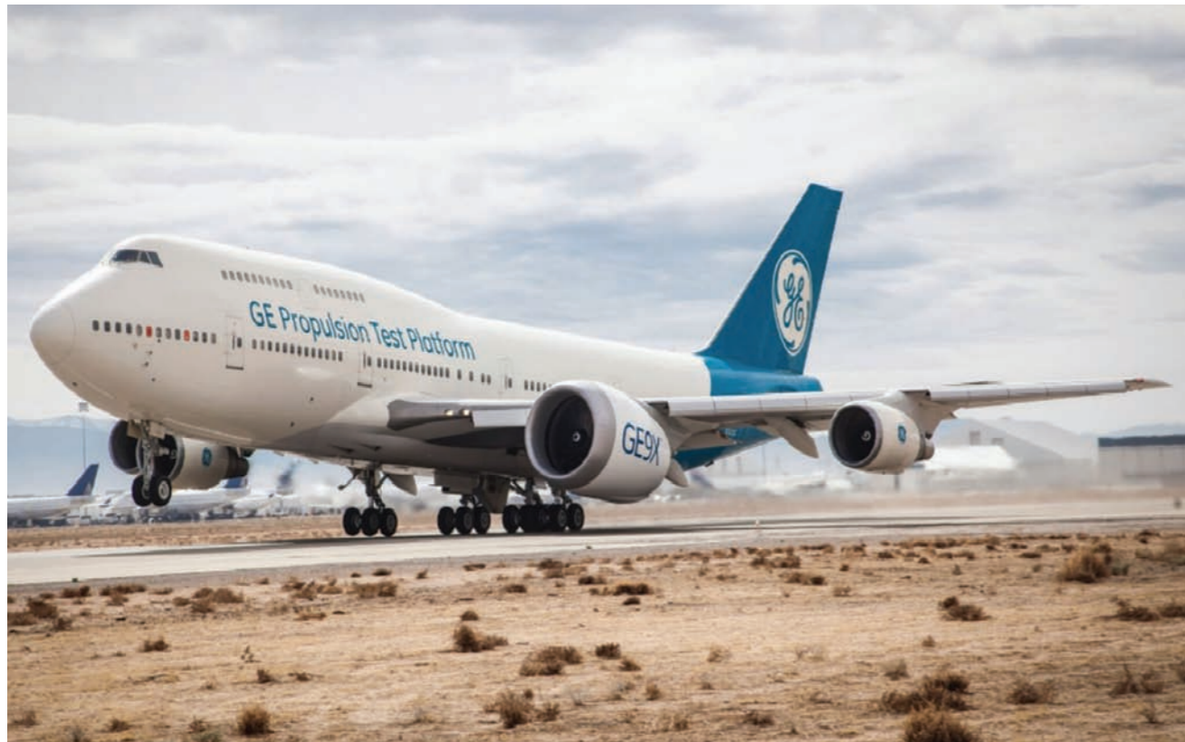
Installing the powerplant on inboard pylon of 747-400 flying testbed's left wing – carried out in record time – was a major engineering feat
