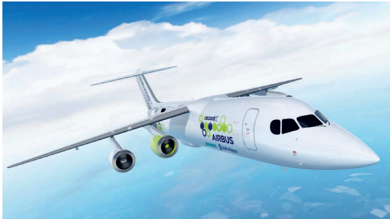
Airbus E-FanX demonstrator will be a BAe 146 adapted to fly on three ordinary gas turbines and one nacelle-mounted electric fan
