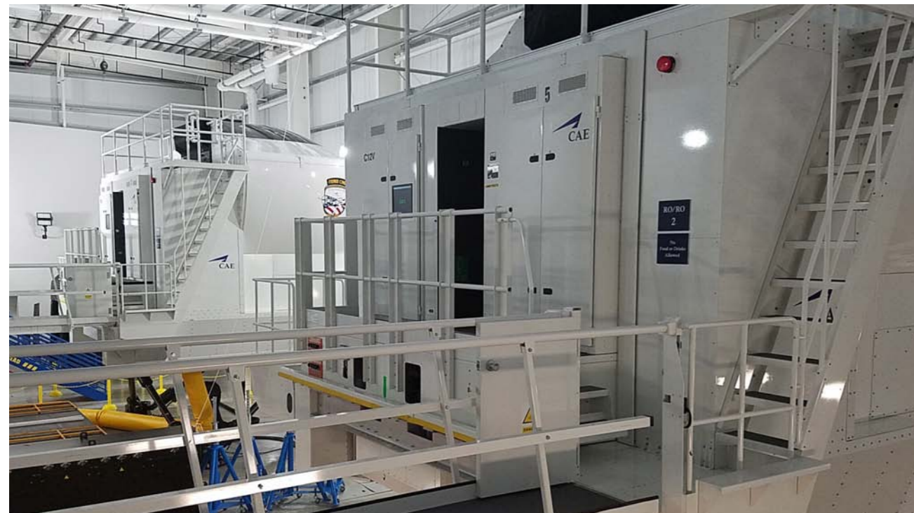
CAE's Dothan Training Center in Alabama houses CAE-built C-12 Huron full-flight simulators to support US Army fixed-wing flight training
