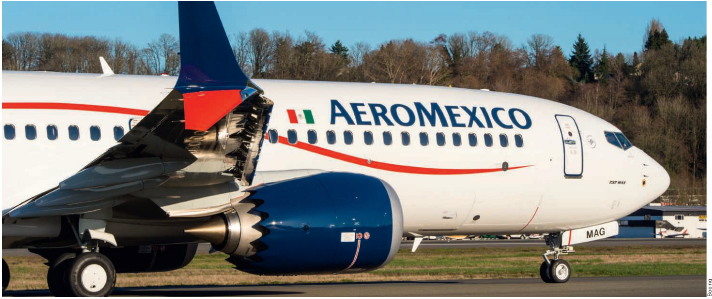
Aeromexico 737 Max 8 shows off the re-engined narrowbody's distinctive split-tip winglets and CFM International Leap-1B powerplants
