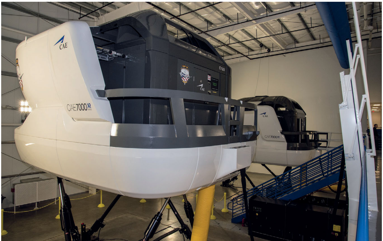
Shown are two of the CAE 7000XR C-12 (King Air) full-flight simulators operated at the CAE Dothan Training Center to support the Army fixed-wing flight training programme
