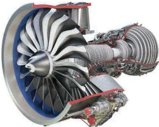
The Leap engine will be the first commercial turbofan to incorporate ceramic matrix composites (CMCs)
