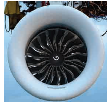
The Leap-1A is one of the three variants of the newest CFM engine
