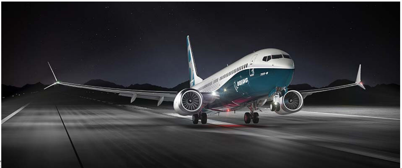
The Leap is the exclusive powerplant on the Boeing 737 Max which will enter service in 2017
