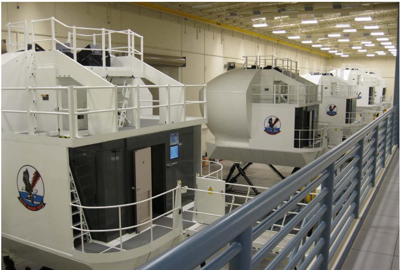
Boeing P-8A Poseidon OFTs operated by the US Navy at the Naval Air Station in Jacksonville, Florida
